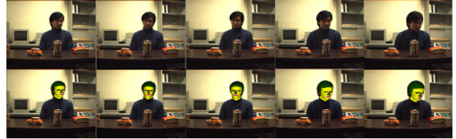
Fig.1: Estimated results of face orientation. Upper: Input images; Lower: Reconstructed face orientation corresponding to its upper image.
